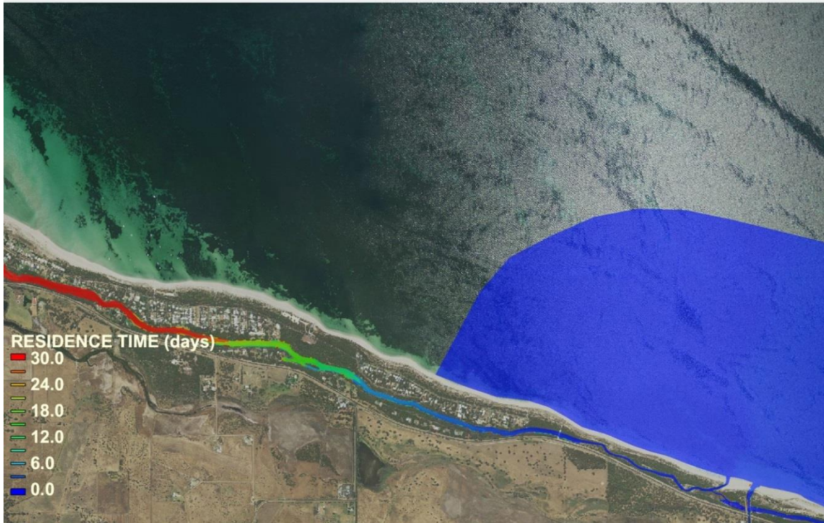
Station Gully closed, Toby Inlet open, culvert open
