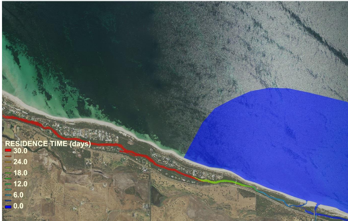
Toby Inlet closed, Station Gully open, culvert open
