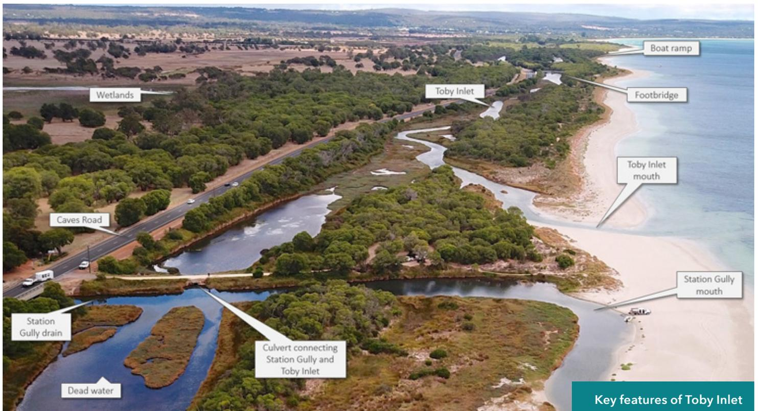
**Maintaining the opening at a height greater than -0.15 mAHD will reduce the risk of the Inlet draining on low tides. The City of Busselton have installed monitoring equipment to monitor the height of the opening over summer.**
